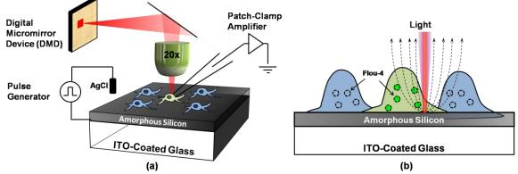
**Fig 1. (a)** Schematics of the optical neural stimulation setup. DMD provides dynamic light addressing capability. The open top design allow patch-clamp recording. (b) Schematics of device operation. Light induces local electric field, which depolarize the nearby neurons. The depolarization causes increase of  $Ca^{2+}$  in the cell, and the event can be monitored by Flou-4 fluorescent intensity increase.
